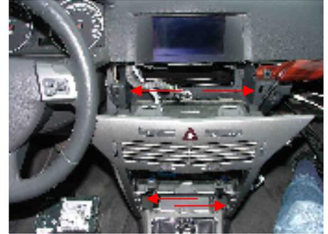
5: Disassemble the 2 torx screws of the CID. Disassemble the screen.
