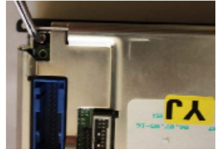
19: After that, you have to screw them until the rear shielded plate is fixed. Insert the torx-screws through both interface holes and screw them into special screws in order to fix the interface to the CID. See picture.
